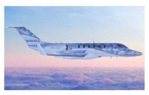
Significantly more passenger space as well as a class-leading cabin tranquility with greatly reduced vibration compared to conventional light jets, due to the OTWEM configuration. The aircraft also has the tallest cabin height, and offers class-leading pressurization with a cabin altitude of 6,363 feet at its max operating altitude of 47,000 feet. Finally, the aircraft will also offer 3 types of modular and highly customizable cabin configurations.
