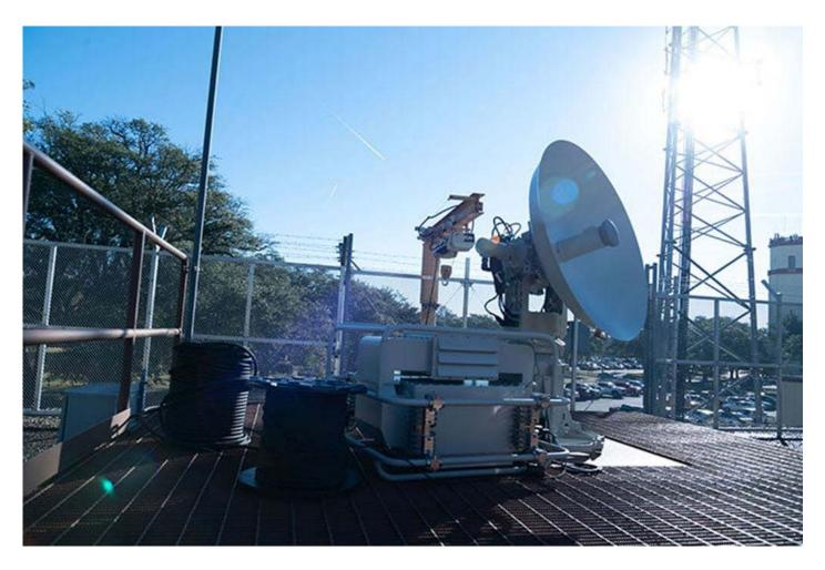
Raytheon Intelligence & Space, a Raytheon Technologies business, completed the installation of the first Global Aircrew Strategic Network Terminal system for the US Air Force. The terminal system modernizes existing protected communications systems while adding new capabilities for nuclear and non-nuclear command and control. Global ASNT ensures robust communications to provide protected communications to nuclear bomber, missile and support aircraft crews in austere environments.
