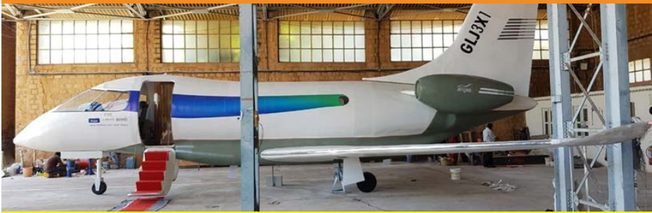
Full Scale Mock up Built at Jakkur Aerodrome Hangar, Bengaluru
